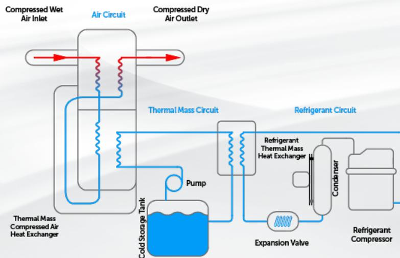
Moisture saturated Compressed Air from the Air Compressor enters a Particulate Pre-Filter then into the Thermal Mass Dryer-Compressed Air Travels through a Coalescing Pre Filter and then 3 in 1 Heat Exchanger.
